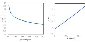
Figure 3 Azeotropic composition of acetonitrile with different pressure
