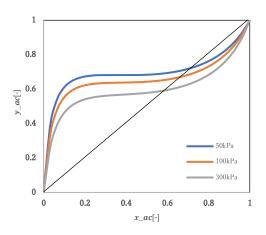
Figure 1 VLE diagram of binary system
