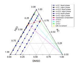
Figure 2 VLE diagram of ternary system
