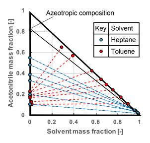
Fig. 1 Phase Diagram of Liquid-liquid equilibrium ternary system
