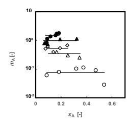
Fig. 2 Distribution coefficient of acetonitrile with solvent of mixture heptane and toluene
