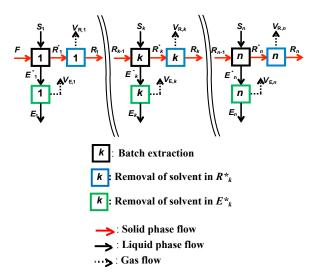
Figure 1 Multistage crosscurrent extraction procedure
