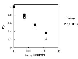
Fig.2 Effect of nitric acid concentration on the Extraction degree.  $C_{La,aq,0}$ =0.1 kmol/m<sup>3</sup>,  $C_{RH,org,0}$ =0.5, 1.0kmol/m<sup>3</sup>
