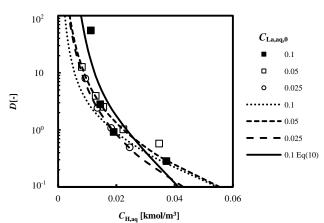
Fig.5 Effect of hydrogen ion concentration on the distribution ratio. The comparison of observed distribution ratio (plot) with predicted distribution ratio (broken and dotted line).
