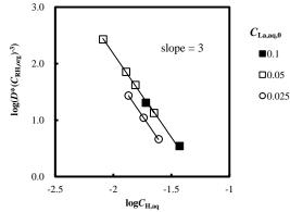
Fig.4 Determination of  $K_{ex}$  by using of slope analysis method.  $C_{\text{RH,org,0}}=0.5$  kmol/m<sup>3</sup>,  $C_{\text{La,aq,0}}=0.1, 0.05, 0.025$  kmol/m<sup>3</sup>
