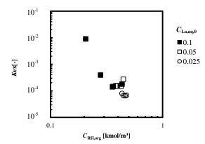
Fig.3 Effect of free extractant concentration on the extract equilibrium constant.  $C_{\text{RH,org,0}}=0.5$  kmol/m<sup>3</sup>,  $C_{\text{La,aq,0}}=0.1, 0.05, 0.025$  kmol/m<sup>3</sup>
