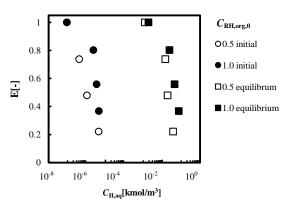
Fig.1 Effect of initial and equilibrium  $C_{H,aq}$  on the extraction degree.  $C_{Laraq,0}=0.1 \text{ kmol/m}^3$ ,  $C_{RH,org,0}=0.5$ , 1.0 kmol/m<sup>3</sup>
