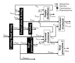
Fig.1 Current and proposed process of sawmilling: material and heat flow
