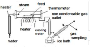
Fig.1 Apparatus of thermal treatment
