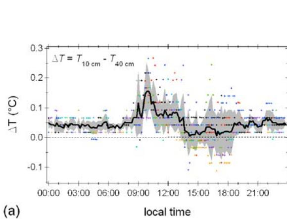
Figure 4: Mean (7 days) diurnal variation in March 2009 of the difference in temperature measured by a HOBO™ mounted 10 and 40 cm away from the actual lamppost, respectively (Velasco 2009, pers. Comm.).
