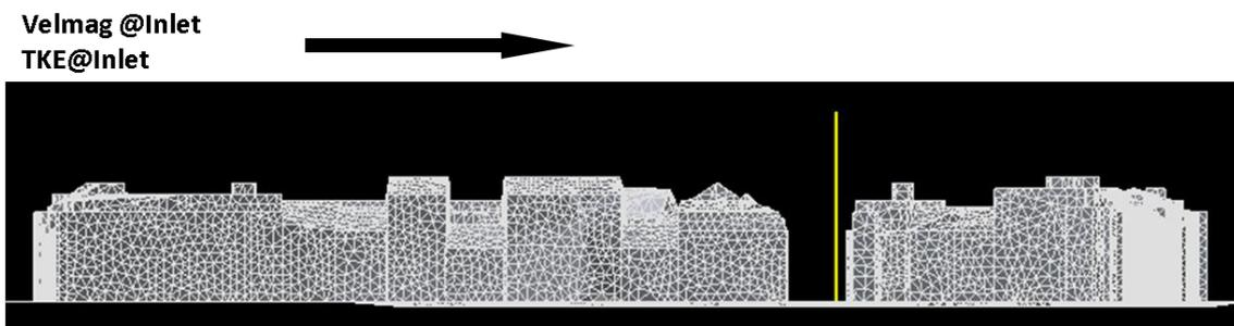
**Figure 1** Cross section through the 3 dimensional mesh, Sperrstrasse, Basel. The line indicates the measurement tower and the arrow the 130° inflow condition
