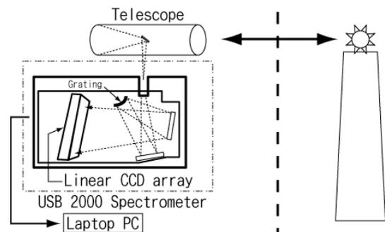
Figure 1. Experimental setup for measuring NO<sub>2</sub>.
