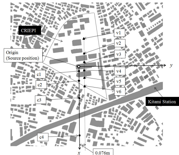
Fig. 2 The locations where the obtained velocity and concentration were observed with the wind tunnel.
