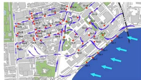
Figure 4: d) evaluation map of air flow pattern in TST
