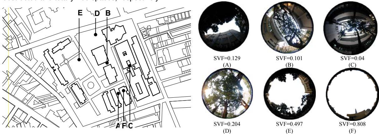
Fig. 1. NFU campus maps and locations of measurement and fisheye photos for each location
