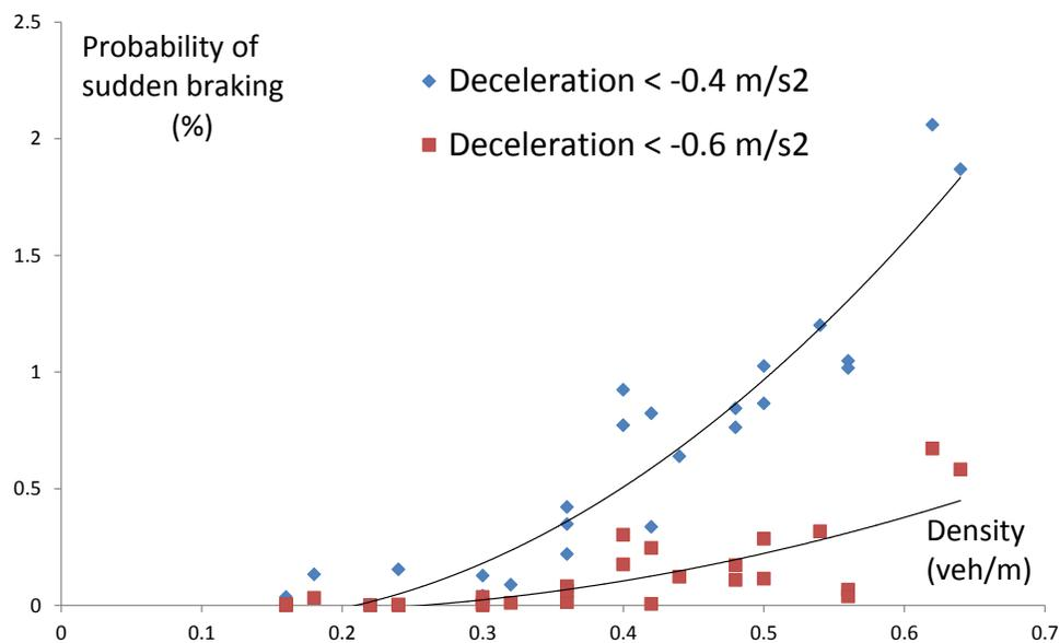
Figure 6.4 Effects of flow density on probability of sudden braking
