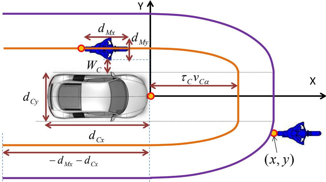
Figure 5.2 Safety spaces for a car when an influential vehicle is a motorcycle
