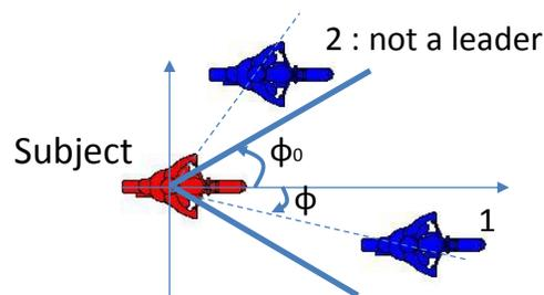
Figure 6.1 The critical following angle of the motorcycle
