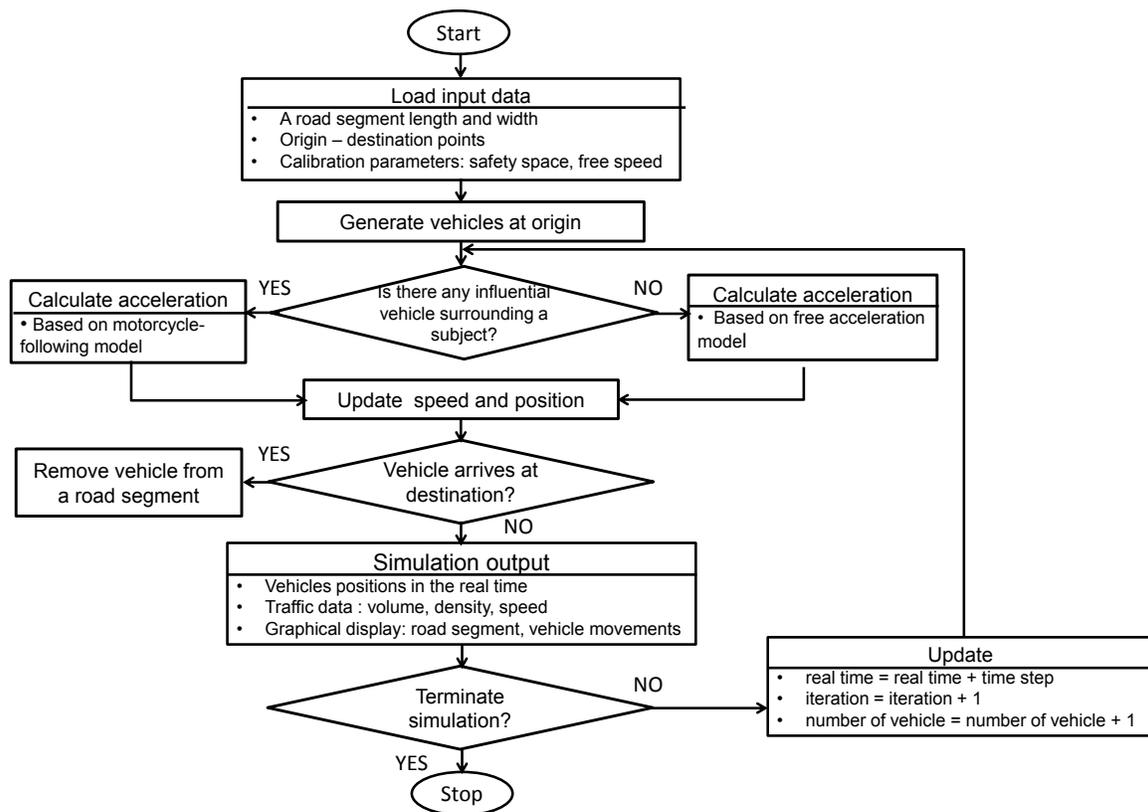
Figure 4.1 Flow chart of the traffic simulation model
