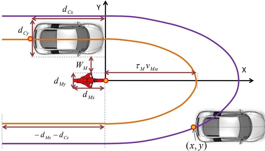
Figure 5.1 Safety spaces for a motorcycle when an influential vehicle is a car
