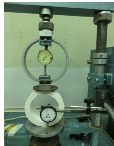
Fig3. Brazilian test of hollow-cylindrical plaster cement in EGAT
