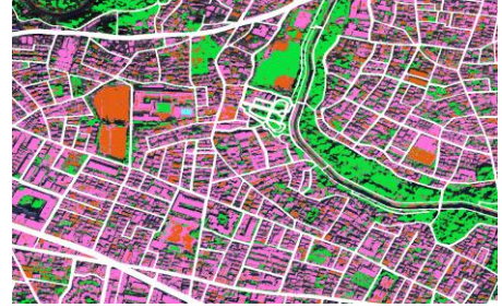
Fig. 6: Result of supervised classification. (Purple: building rooftops, Green: vegetation, Orange: bare lands. Road faces are whitened using ESRI data)
