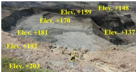
Fig. 1 Actual practice of undercut slope at the Mae Moh lignite mine in Thailand (as of October 2012)
