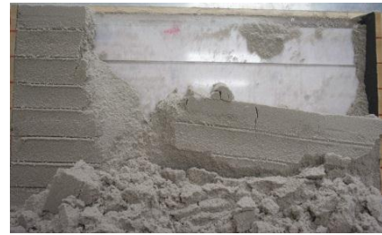
Fig. 7 Collapse of undercut slope in a buckling mode of Test 5
