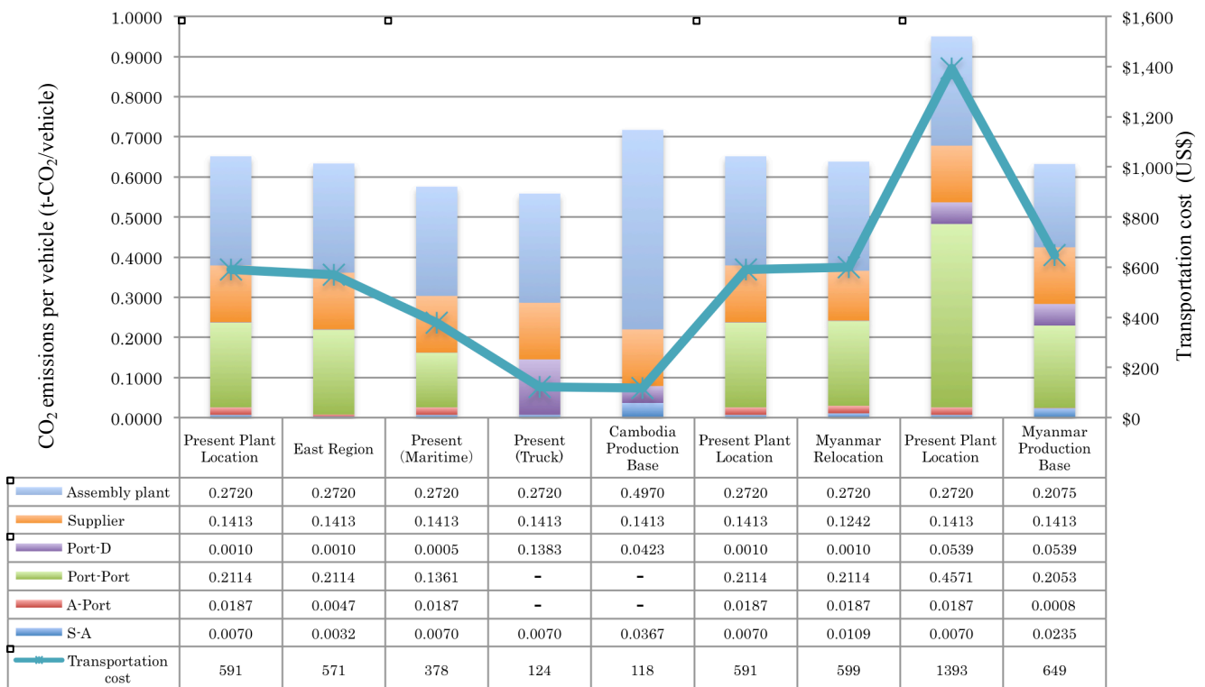
Fig.6 CO 2 emissions results (S: Supplier, A: Assembly Plant, D: Distributor)
