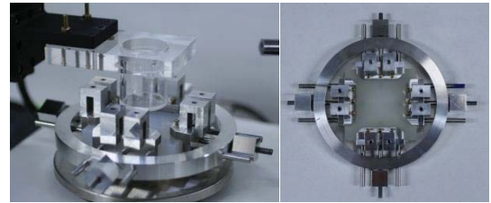
Figure 3 Photographs of Generator of circumferential strain of disk surface (fig 2(b)) : GCD and Lens fixing base (fig 2(a)) : LFB.
