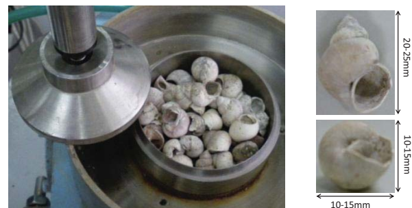
Fig. 2 Specimen of snail fossil in oedometer tests
