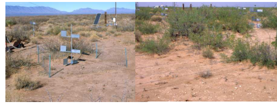
Fig. 7. Photograph near the sand trap station in JER taken in December 2001(left) and May 2002 (right). Note that even without leaves, shrubs can be enough obstacle for sand transportation.
