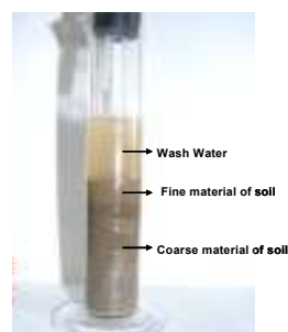
Fig. 6 Two layers of sediment after agitation
