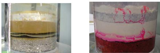
Fig.16 OC Hachioji loam Fig.17 NC kaolin with ink
