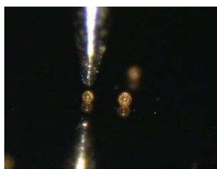
FIG. 6. Photo obtained before micro-particle pickup.
