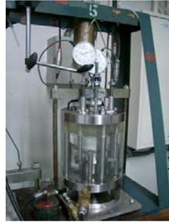
**Fig.8**  $K_0$  apparatus
