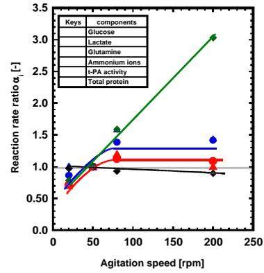
**Fig. 3.2.** Effects of agitation on (a) specific growth rate ratio,  $\alpha_{\mu}$  [-] (above); (b) reaction rate ratio,  $\alpha_i$  [-] (below).
