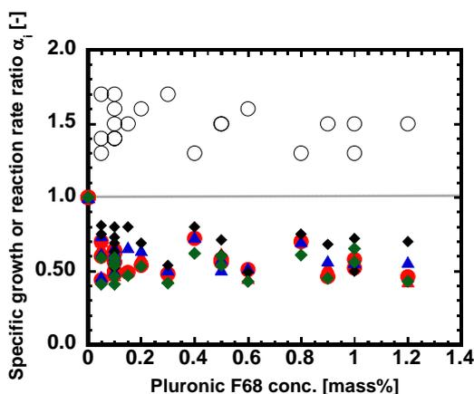
**Fig.3.3.2.** Effects of Pluronic F68 addition under static conditions : (  $\circ$  :  $\alpha_\mu$  [-]; the others are the same as Fig 3.3.1.(b).)
