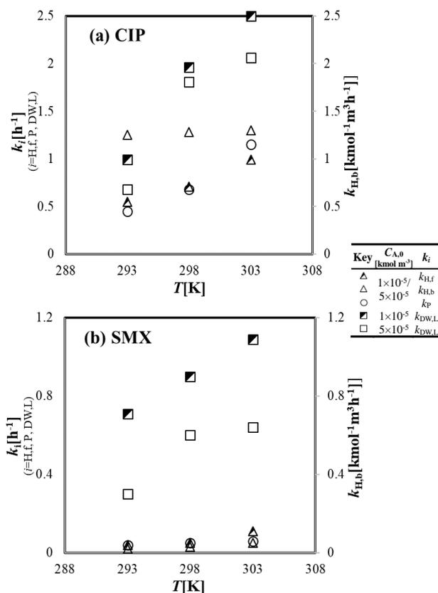
Fig. 2 The reaction rate constants for each antibiotics removal mechanism under different temperatures
