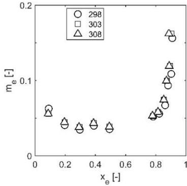
**Figure 4** Relation of mass ethanol in feed with ethanol distribution coefficients
