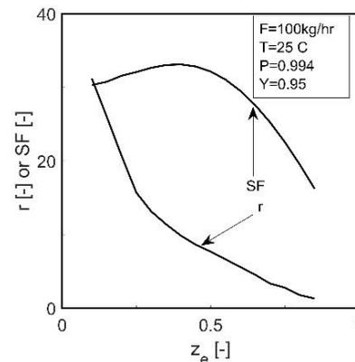
Figure 9 Correlation of mass ethanol in feed with reflux and solvent per feed flow ratio
