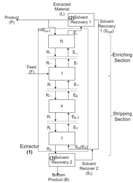
**Figure 6** Schematic diagram of a countercurrent multistage extraction
