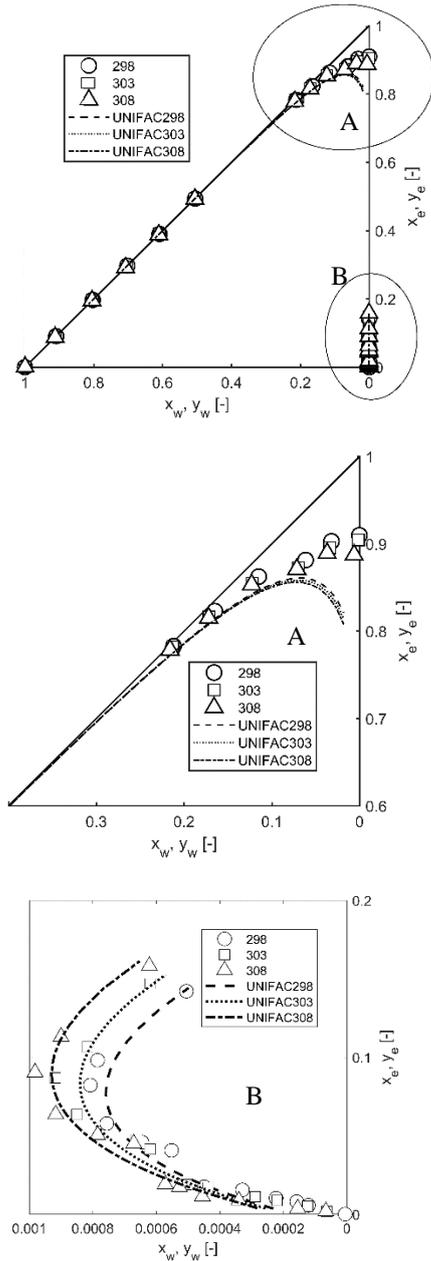
Figure 2 Liquid-liquid equilibrium in different temperature (A) raffinate phase (B) extract phase
