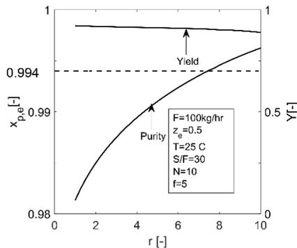
Figure 7 Effect of reflux ratio to product purity and yield
