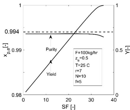
Figure 8 Effect of  $S/F$  flow ratio to product purity and yield
