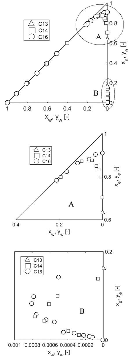
Figure 3 Liquid-liquid equilibrium in different solvent (A) raffinate phase (B) extract phase
