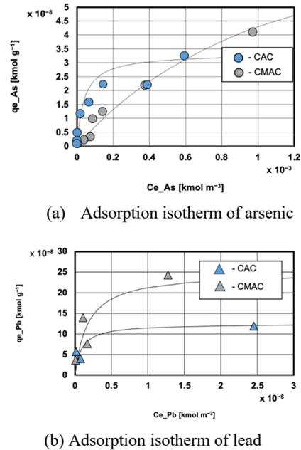
Fig. 6 Adsorption isotherms of single component adsorptions of As and Pb
