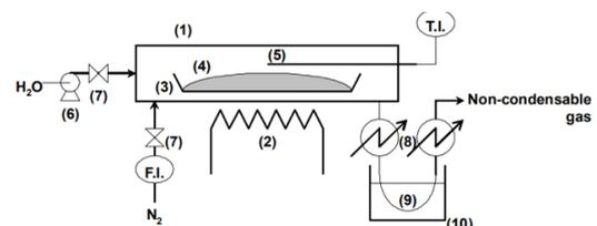
Fig. 1 Thermal treatment reactor
