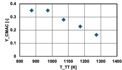
Fig. 2 Effect of thermal treatment temperature on yield
