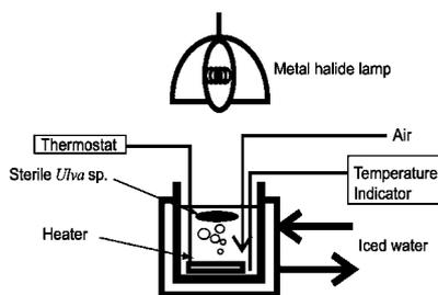
**Fig. 1** Experimental apparatus (stainless steel tank)
