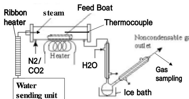
Fig.2 Experimental equipment
