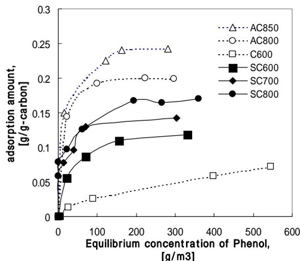
Fig.4 Adsorption isotherms of phenol in model solution at 30 °C on the different carbons ( , , [3])
