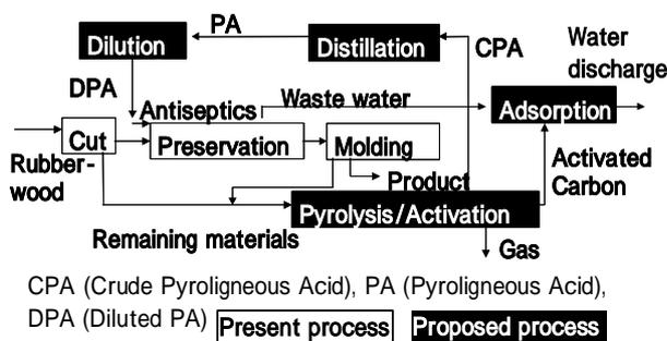
Fig.1 Schematic diagram of rubberwood process
