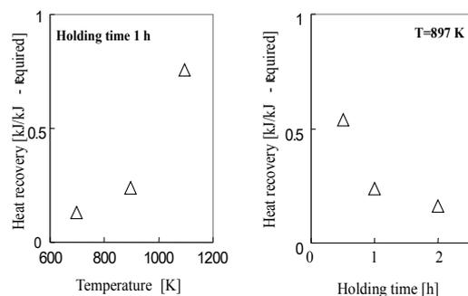
Fig.4 Heat recovery of off-gas
