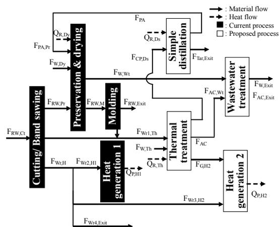
Fig.1 Current and proposed process of sawmilling: material and heat flow
