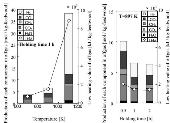
Fig. 3 Production of component of off-gas
