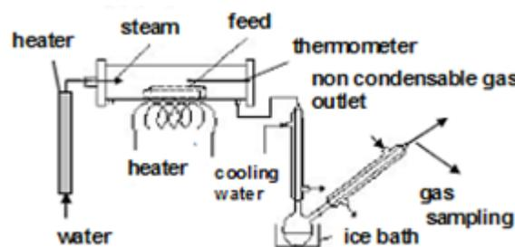
Fig.1 Apparatus of thermal treatment
