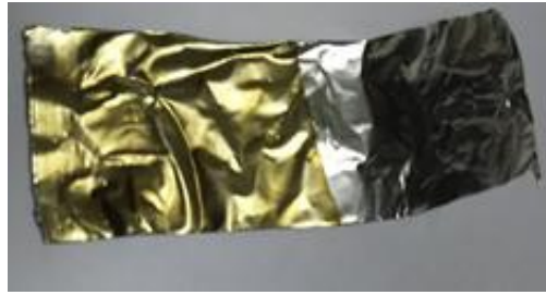
Figure18: Al sheet coating with GO
